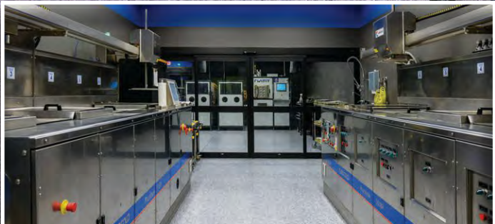
TWO advanced robotic EUROCOLD Pluritank® cleaning systems, removes oils and contaminants from tools prior to coating.
