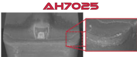
Tool wear after 60 grooves
