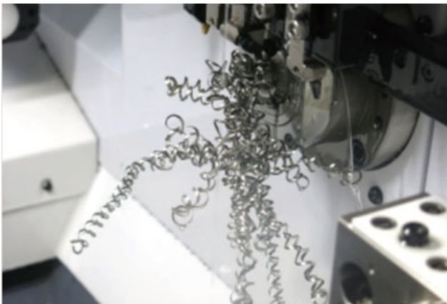
External coolant supply at normal pressure
