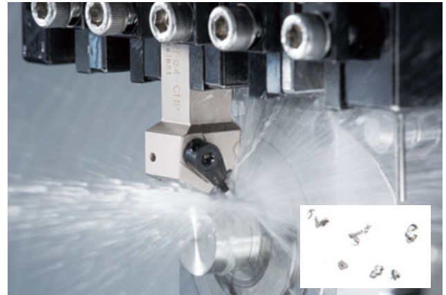
High pressure coolant (7 MPa)
