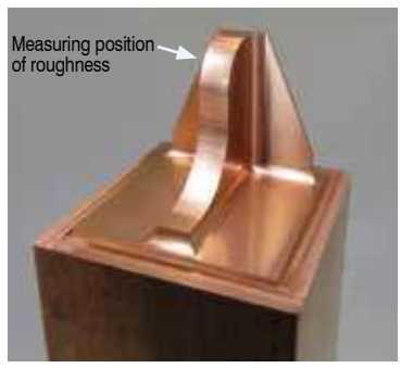
Model Size : 20 x 20 x Depth 16 mm Coolant : Oil Mist
