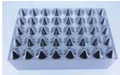
Work Size : 80 × 50 × 30 mm Coolant : Oil Mist
