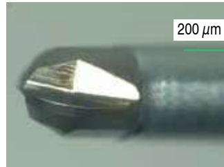
Tool damage after 10 hours of milling.
