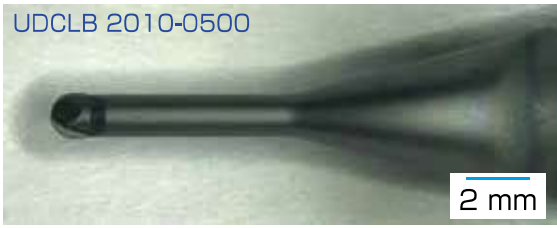
Tool #2 milled 131.9 mm 3 in 76.5 minutes.
