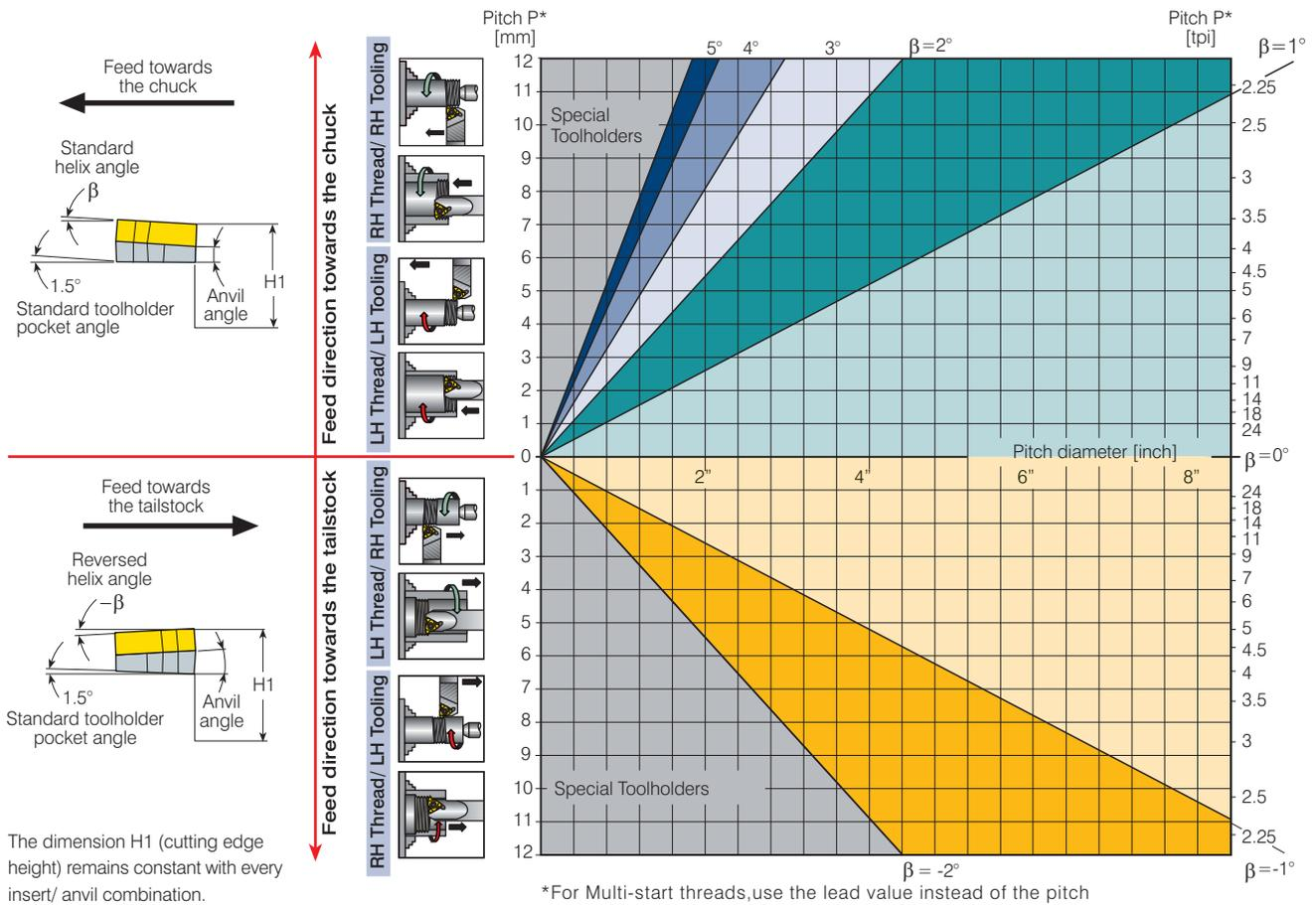
The dimension H1 (cutting edge height) remains constant with every insert/ anvil combination.
