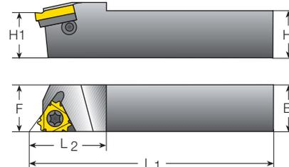
V6 inserts can be used on any External RH holder that uses an anvil.
