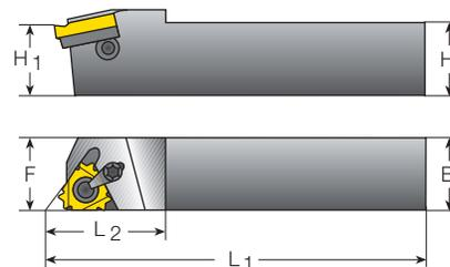
V6 inserts can be used on any External RH holder that uses an anvil.
