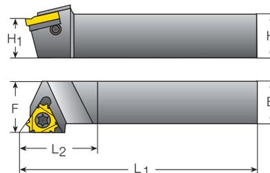
V6 inserts can be used on any External RH holder that uses an anvil.
