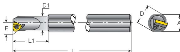
V6 inserts can be used on any Internal RH holder that uses an anvil.
