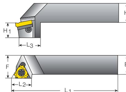
V6 inserts can be used on any External RH holder that uses an anvil.
