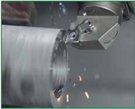
Insert with Chipbreaker
