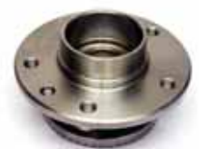
Hub Roughing and Finishing
