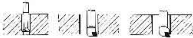
Boring with several different bits from \varnothing 0.5 – 1250 mm
