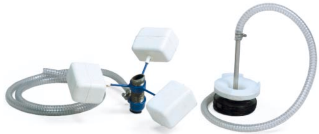
A float-type suction device is included as standard (left). The optional bellows type (right) is designed for narrow spaces and shallow tanks (up to 100 mm).
