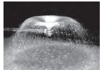
At 1 p.s.i.: Wide spray angle with large droplets and minimal misting.
