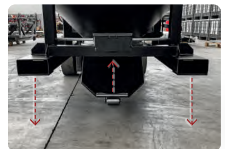
Door closing system by pressure on the floor.
