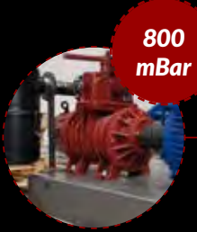
High Vacuum Pump with 800 mBar depression
