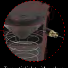
Tangential inlet with cyclone
