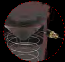
Tangential inlet with cyclone
