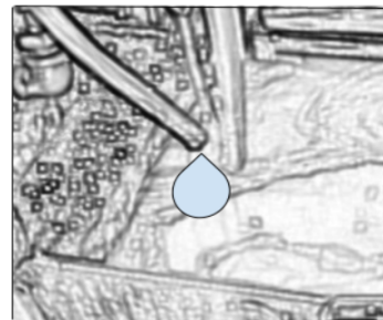
Cut off the excess tubing leaving it at least 3" above the coolant level in the tank.
