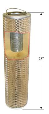
A Large And Structurally Strong Cartridge With 42 Square Feet Of Filter Surface To Allow Up To 30 Lbs. Of Solids Holding Capacity. This Cartridge Can Be Used On Process Water And Oil Fluids. (Not To Be Used On Potable Water.)
