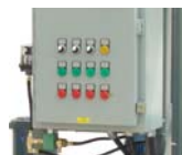
Nema 12 electrical enclosure; with IEC Controls, with Rotary Disconnect. 230 or 460 Volt Three Phase
