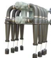
The Ebbco Cyclone filter is designed to separate foreign particles from liquids—centrifugal force generated in a cyclonic chamber at 20 gpm each. Providing 10 micron clarity
