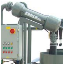
The Centrifugal Separator is constructed of Carbon Steel, Designed To Remove 98% Of Particulate From Liquid, With A Specific Gravity Of 2.6 Or Higher. Separator Is Sized To Filter to 30 Micron Clarity
