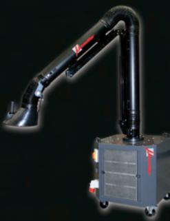
The new QUAD with its small size and versatility provides a definitive solution to the problems of fume removal. The QUAD provides filtration and deodorization of fumes, solvent and aerosols. It is suitable for many various manufacturing processes: welding, EDM, induction machines, blocking tool machines and for all applications where any type of dry smoke or odor is being created. The QUAD is equipped with 4 wheels for easy portability and the Evolution arm.
