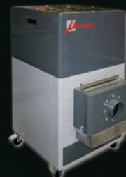
SHARP filter unit has been designed for all applications where dry sharpening, grinding and similar activities are the core of the metal working process. The SHARP is designed so that no sparks from the grinding process are allowed to reach the filter media. Easy to handle and versatile, the SHARP is available with three different electric motors 0.75 kw, 1.1 kW and 2.2 kw (1 HP, 1.5 HP and 3 HP) and can be equipped with suction arm and also with final HEPA after filter.
