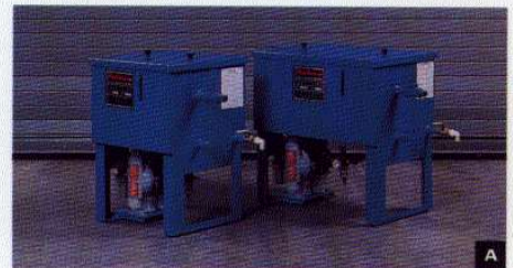
THE MINI AND JUNIOR DEDICATED SEPARATORS PROCESS SUMPS FROM 40-200 GALLONS.
