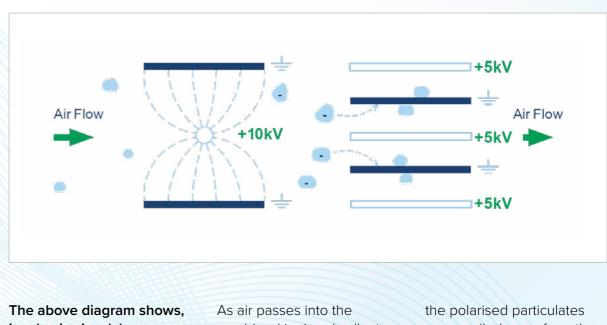
in a basic visual, how an electrostatic precipitator works:
