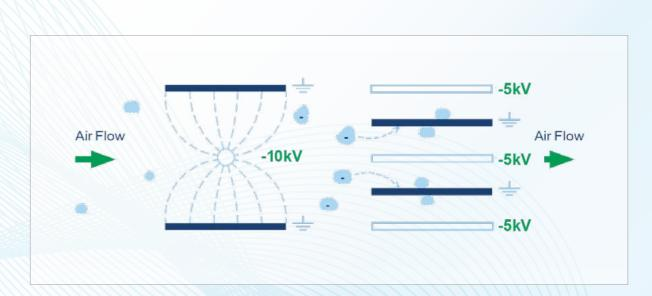
The above diagram shows, in a basic visual, how an electrostatic precipitator works: As air passes into the combined ioniser / collector cell, the particulates in the air stream are polarised. As they continue through the ioniser and between the collector cell plates,
