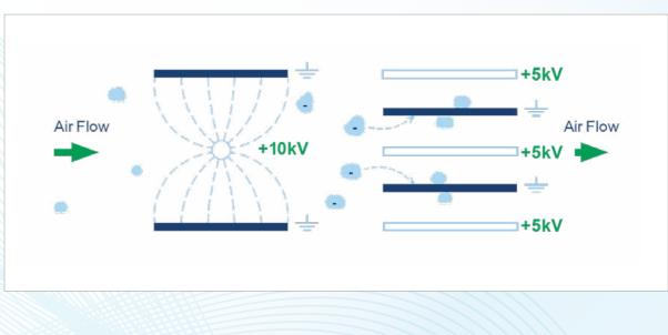
The above diagram shows, in a basic visual, how an electrostatic precipitator works:
