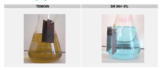
5.1.1.2. <u>MEASCOVN03 method</u>: "Effectiveness of an anticorrosion additive on cast-iron swarf". (based on DIN 51360-part2)
