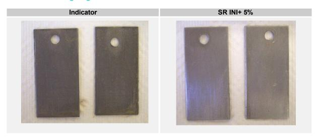
5.1.2.2. <u>MEASCOVN03 method</u>: "Effectiveness of an anticorrosion additive on cast-iron swarf". (based on DIN 51360-part2)
