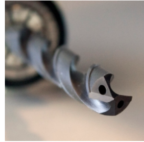
Figure 21: Thru-the-tool exit holes
