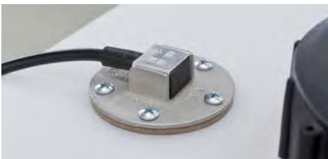
Level sensors monitor fluid levels
