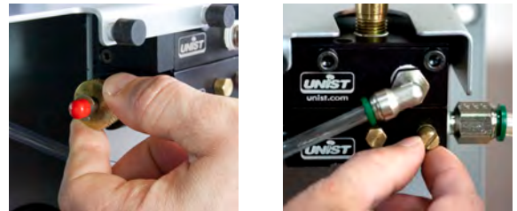
Easily adjust pump stroke and air flow for the perfect spray.
