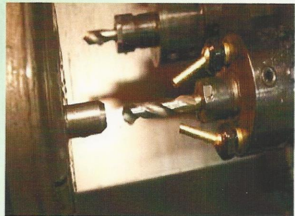
DUAL THREAD-JET ON CNC LATHE DRILLING OPERATION, WITH 32MM EXTENSION TUBES
