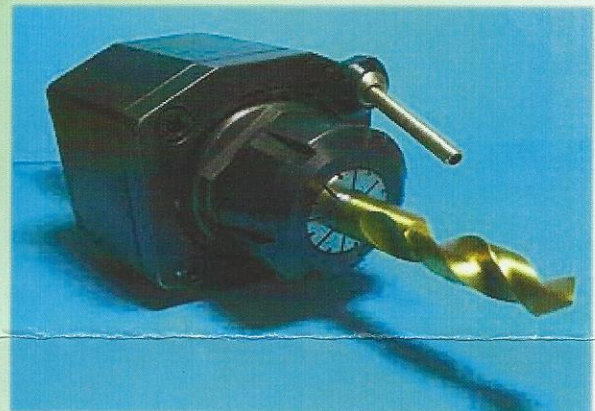
THREAD JET SHOWN ON VDI LIVE TOOL WITH 44MM EXTENSION TUBE.
