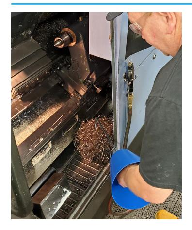
The new design provides a simple, solid method to remove chips from hazardous and hard to reach areas. Second generation chip hook features a large cone which offers protection for the entire hand, single or double-handed handles available. Bright blue color guarantees high visibility and wooden handle ensures a firm grip.
