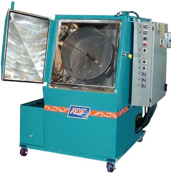
Rinse machine shown with optional recirculating rinse tank and hot compressed air blow off. Basket lid not shown.
