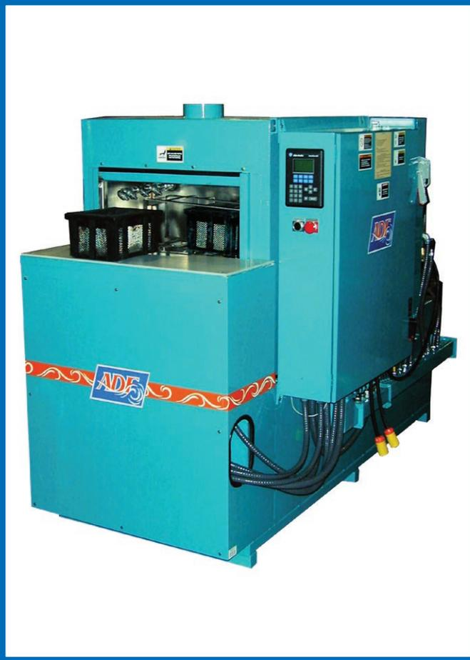
The Model 750 Rotary Basket Parts Washer is designed to clean parts that are best suited to being tumbled, rotated, immersed, and sprayed for proper cleaning. It offers the cleaning system needed for parts with blind holes, internal holes, cavities, threads, and those small parts that tend to nest preventing total cleaning. The hydraulic action of the fluid entering and evacuating the cavities offers excellent cleaning and rinsing.
