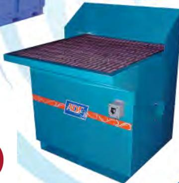
The open mesh table draws air and contaminants like grinding dust welding fumes and smoke away from the operator.
