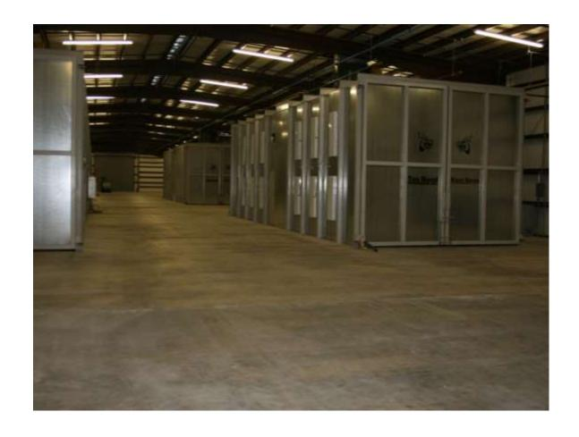
Seven booth installation, all 16' wide x 14' high x 50' long 2 – Blast Booth , 5 – Paint Booth (one with heated air make-up)
