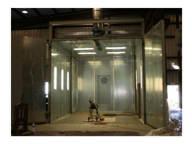
Swing style doors cover the paint plenums when in blast mode, swing to the rear wall to expose the paint filters for paint mode.
