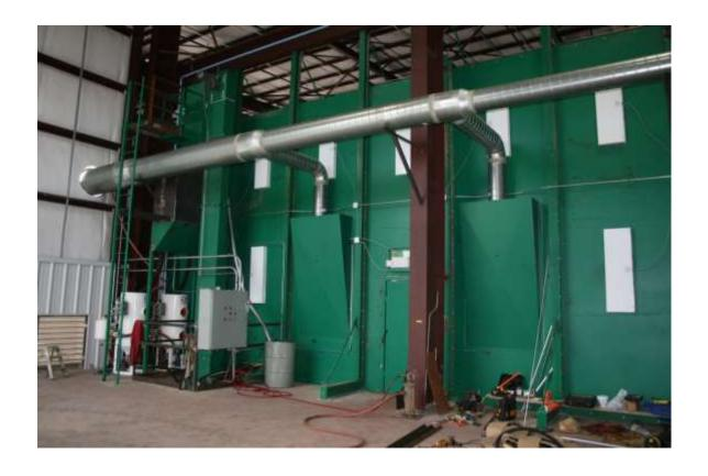
Reclaim system for single screw cross auger w/ dual outlet storage hopper. Hopper was expanded in the field at the customers request.
