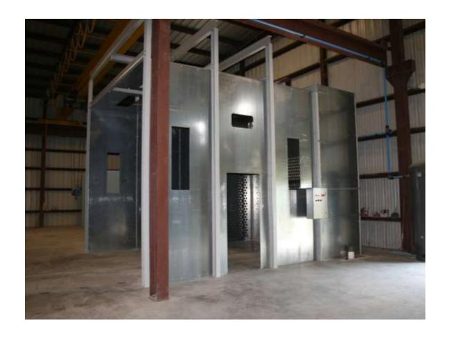
16' wide x 14'-6" high x 20' deep combination blast and paint booth under construction. New design with galvanized sheeting.
