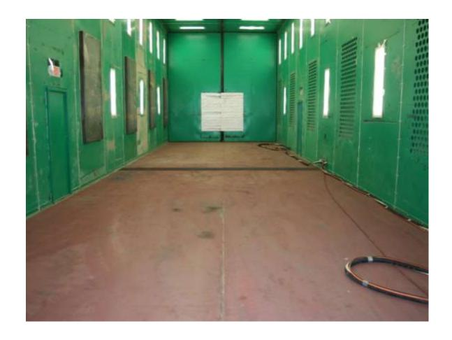
Interior view with single cross auger recovery. Note the finger seals added in the product door. This was added in the field to accommodate 100' riser sections.
