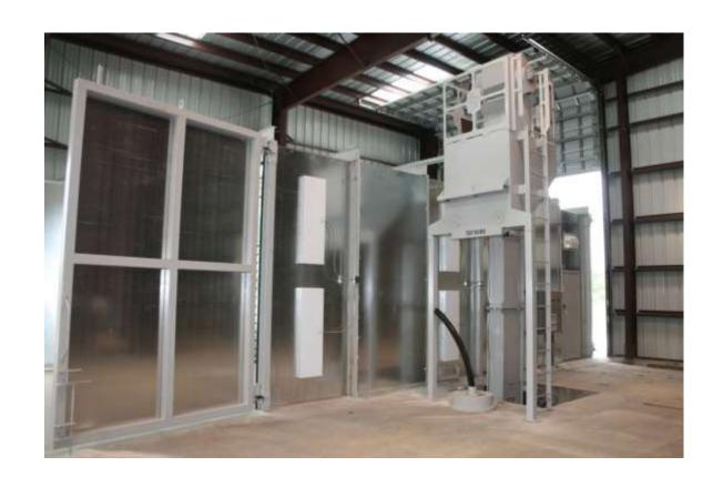
New Design – Reclaim Unit Modular design, 55 cu. ft. dual outlet storage hopper
