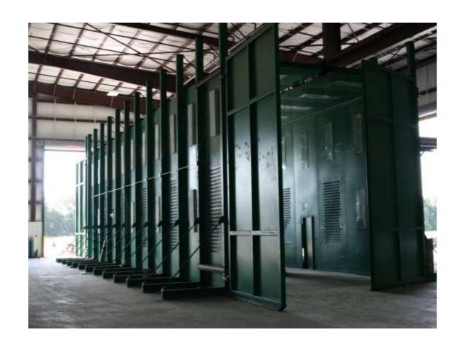
$20' \times 20' \times 70'$  – Full Slot Seal Booth Cross Flow Design (left side of booth inlet air / right side connected to D/C
