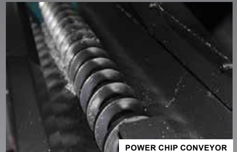
POWER CHIP CONVEYOR
