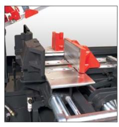
Indexing accuracy of  $\pm$  0.004" / index. Both vise jaws open on the indexing vise to accommodate crooked bars and to eliminate scoring the OD of finished bars.
