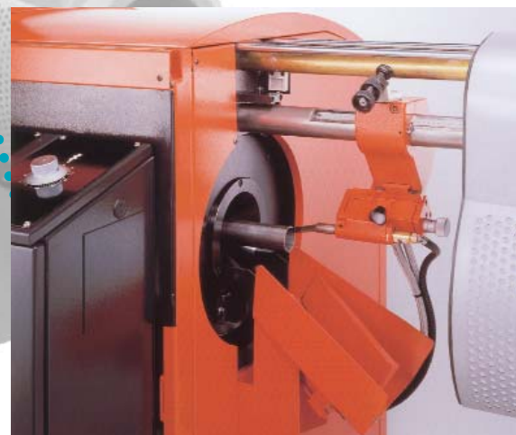
LENGTH STOP Graduated length stop for fast accurate set-up and change over.
