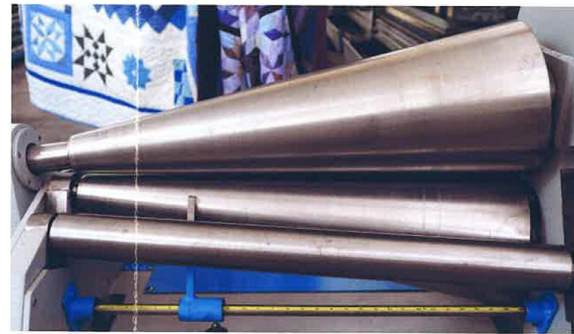
In feed area, notice work piece location pointer
