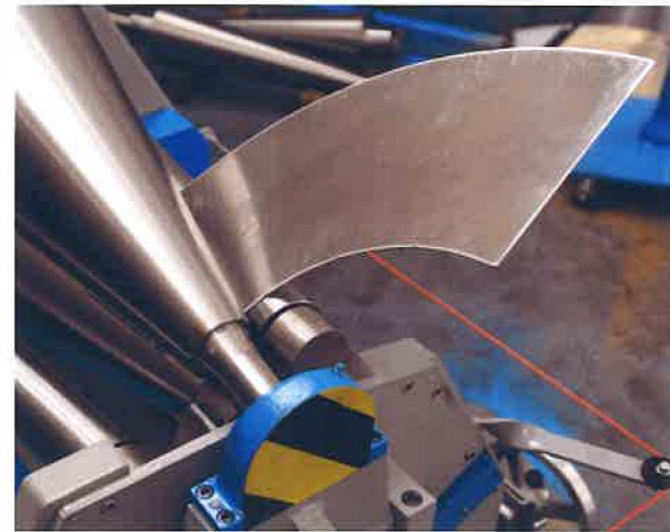
Near forming roll is raised to form leading edge. Rolls rotate to complete bend.
