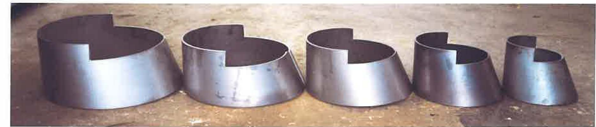
Notice the forming quality of these straight sided asymmetrical cones
