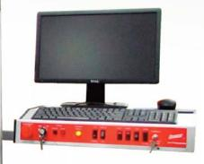
User-Friendly control panel on convenient double-jointed swinging arm.
