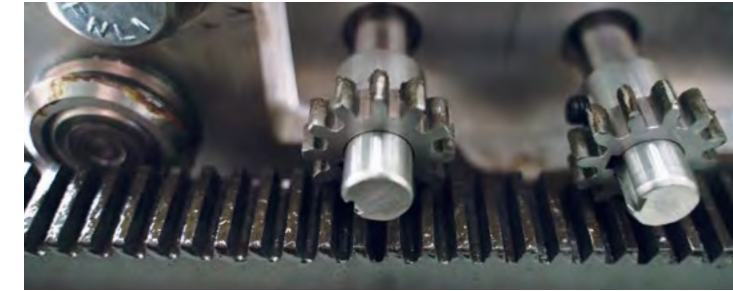
X-Axis: A precision rack and anti-backlash pinion drive system moves the material along its length.
