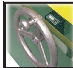
The Optional Front Reading Manual Backgauge Features an Attached Meter, Clearly Indicating Where the Gauge Bar is Located in Relation to the Die.
