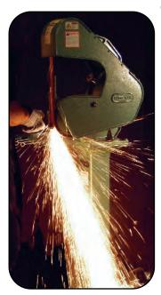
Contact wheel grinding is the most aggressive type of grinding and should be used when heavy stock removal is required. Each elastomer tired aluminum contact wheel is precision machined and balanced for smooth operation. It has been said, when compared to a bench grinder, "that grinding on a Burr King is like grinding on velvet." The contact surface is bonded neoprene, available in 55 and 90
