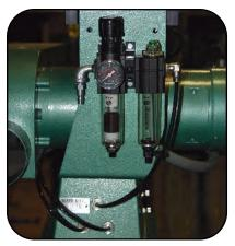
The Model 720 presents a unique up front, two wheel, rear drive configuration that quickly accepts contact wheel finishing diameters from 3/8 inches to 3 inches in diameter. The Model 720 is equipped with a reliable and fully adjustable air pressure, belt tension control system. Using 1/2 inch to 2 inch belt width. The Model 720 72 inch belt track delivers long abrasive life coupled with excellent utility. Available in single or Vari speed. See page 13 for accessory arms.
