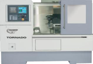
**3-Axes Turning & Milling** Have a fully programmable 'C' axis and power driven tools for radial and axial milling, drilling, boring and tapping.
