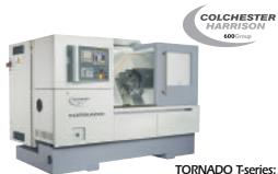
CNC Slant Bed Lathes offer Chucker, Bar and "Lights Out" models, with a Fanuc 21i control on 2 axes and 3 axes with live tooling models, and Fanuc 18i control on 5 & 6 axes sub-spindle models. Equipped with 12 station bi-direction turret.
