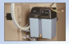
Spray mist coolant unit for FA350A SA and FA350A models. Smaller spray mist coolant units furnished with CA350 and CA350PV. Flood coolant system furnished on all steel cutting machines.
