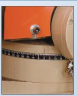
Clearly marked scale to help the operator set-up angle cuts with preset stops at 45° R, 45° L and 0° on manual, pneumatic vise, and semiautomatic models, 45° R, 15° L and 0° on automatic models.
