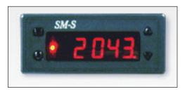
The LCD Display allows the operator to select spindle speeds quickly and accurately. (Not available on models with Programmable Spindle Speeds)
