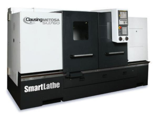
The Clausing/Metosa SmartLathe is designed to handle a wide range of applications, shaft and bar machining, taper turning, thread cutting and much more, with features found on only higher priced machines.
