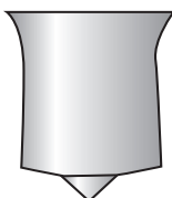
"Y" Shear with Center Point
