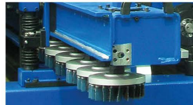
XVS Ø 130 mm with abrasive inserts for deburring and edge rounding
