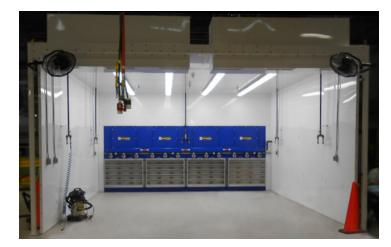
Diversitech's Dust Control Booth are designed to safety capture and filter airbone contaminants from metal finishing, fiberglass, composites and metal fumes.
