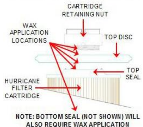
Figure 4.3 Filter Cartridge Assembly Wax Points
