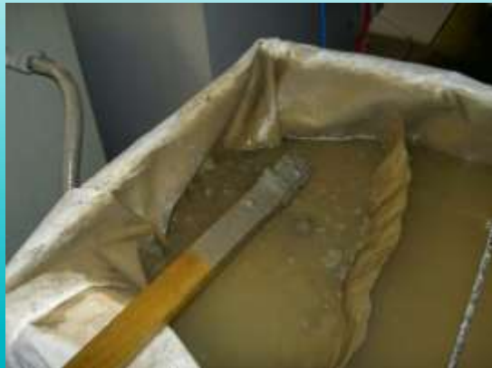
Weir Bag Allows Settlement of the Abrasive Before Entering Closed Loop System
