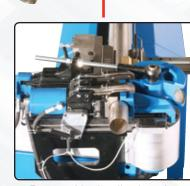
Patented hydraulic clamping system minimizes distance between bends.
