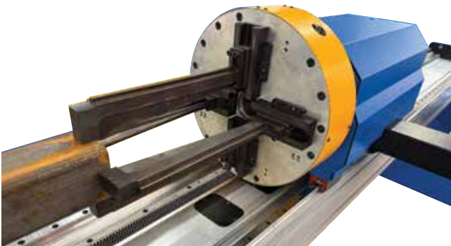
Innovative recessed front gate allowing carriage to position last cut of only 6"
