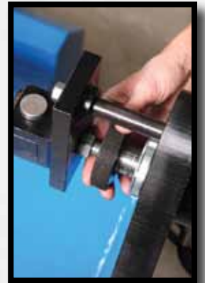
Quick change tooling for easy setup and adjustments.
