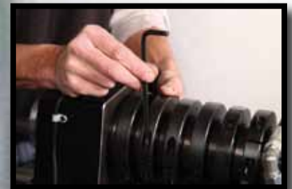
Mechanical stops for distance between bends and rotation from original bend plane.
