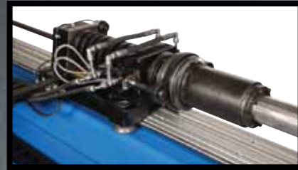
Automated programmable hydraulic clamping secures material in tail stock.
