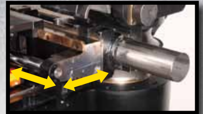
Programmable X2, Y2 axis pressure die movement.
