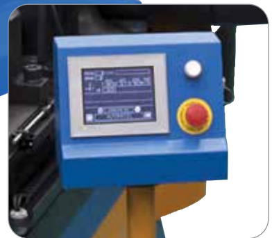
Easy touch screen bend angle programming.
