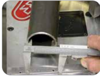
Pipe dimensions are based on I.D. of material (2" sch. 40 pipe measures 2.375" O.D.).
