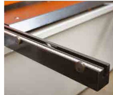
Squaring arm. Makes it easy to handle the work and feeds the material through the cutting area by providing more delicate and quicker cuttings.
