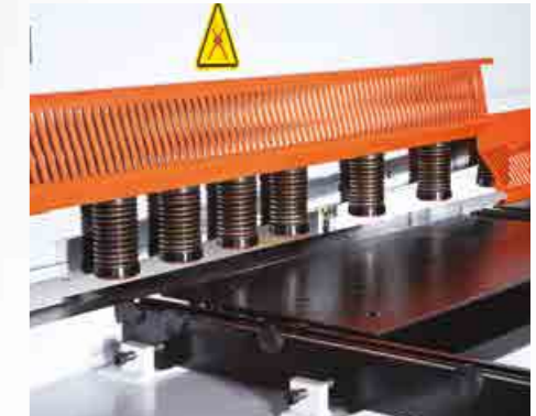
Collapsible finger protection. (standard) In order to control angled cuttings and drawn lines front part of protection can be pulled up by operator. (Switch protected)
