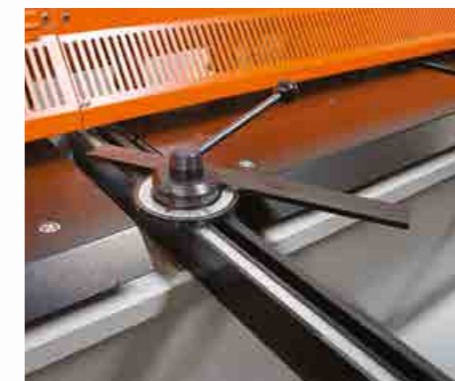
Angle gauge. (option) This device provides accurate and easy material handling in the angled cuttings.
