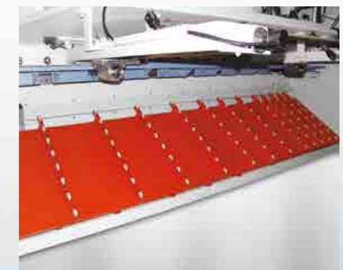
Monobloc type pneumatic sheet support system (optional) Avoids hanging down the wide and thin sheets via pneumatic table support and provides more precise cuts.
