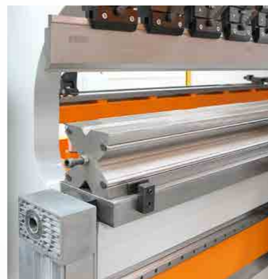
Throat (O) Special throat depths are offered up to 1500 mm for large bends.
